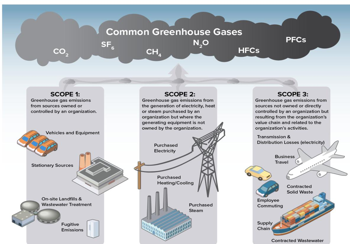
Figure 1. Common Sources of Emissions by Scope
